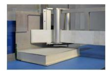
Step 2: The book is drawn along the conveyer belt and an RFID tag is applied automatically
