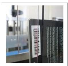
Step 1: The item's barcode is scanned by the integrated barcode scanner
